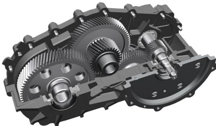
To speed up a transmission gearbox to 20,000 revolutions per minute in a controlled manner is an engineering challenge of its own kind, with complexities like noise, vibrations, frictional power losses, and not the least power losses caused by the viscosity of the lubricating oil.
